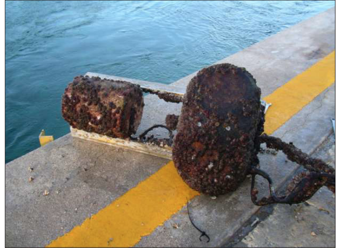
Figure 6a. Acoustic profiler and battery pack after removal from the Boynton Inlet following a 33-day deployment.
