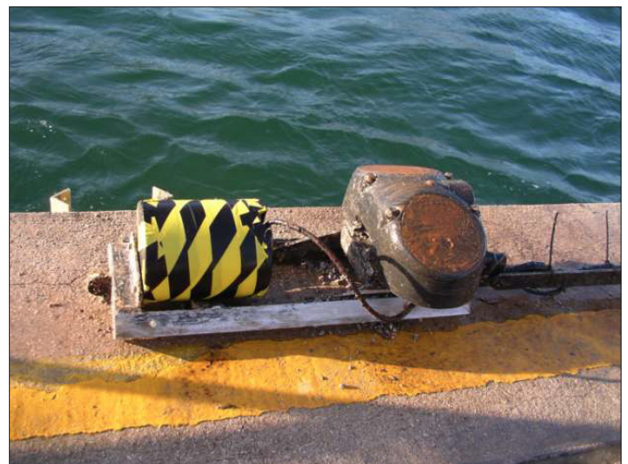
Figure 6b. Acoustic profiler and battery pack after refurbishment and prior to redeployment. Note the mixture of silicone grease and hot chili powder used on the instrument to slow the growth of fouling organisms.
