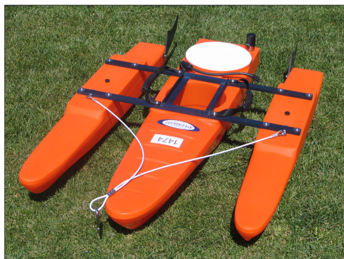
Figure 8. An Oceanscience riverboat system similar to the one used to collect calibration data inside Boynton Inlet.
